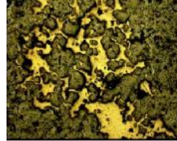
Fig.18- Open-space filling Cpy
