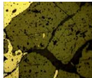
Fig.15- Inclusion of Cpy Inside magnetite
